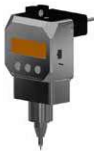
Shore D / C / DO for specialty parts testing
