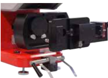
Heating system, ambient to +100°C
