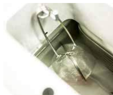
Sample holder in chamber (lid open)
