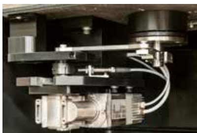
Rheometer brushless DC drive upgrade
