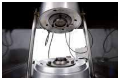
Die upgrades including precision heaters and probes
