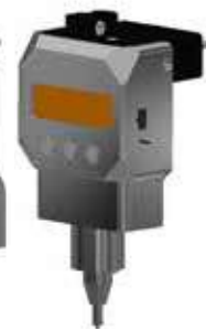
Universal Force / Load Testing with 10N or 50N loadcell
