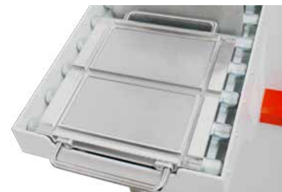
Two cavity sheet mould (2x 200x95x2mm)
