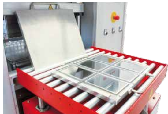
Six cavity sheet mould (6x 150x80x2mm)
