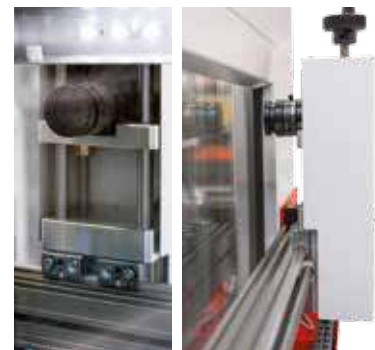
CCD Camera system for crack-growth measurement
