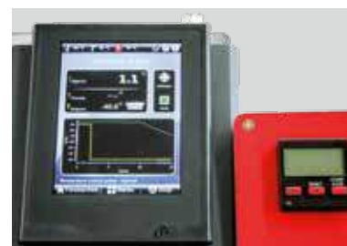
Temperature control touchscreen and timer display
