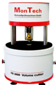
R-VS 3000 constant volume sample cutter
