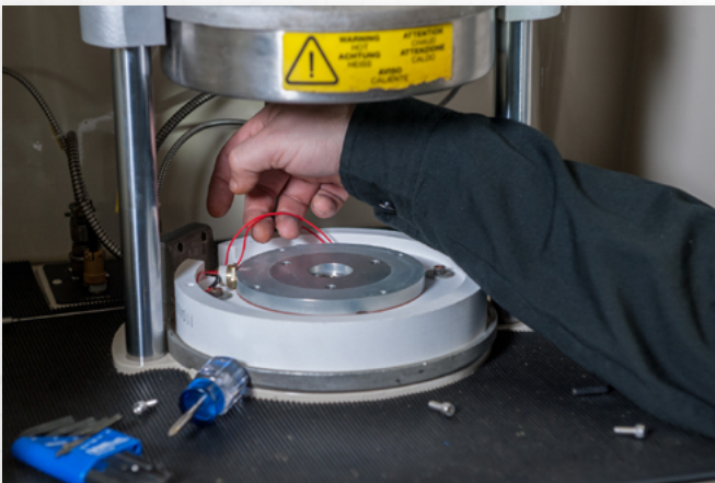
Inspecting Heater Wiring in Lower Platen
