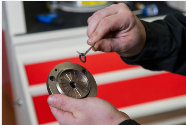
Replacing O-Ring in Lower Platen Die
