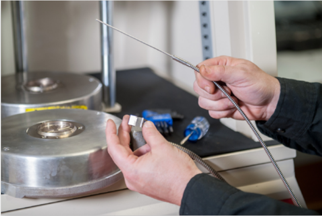
RTD and RTD Clip After Removal
