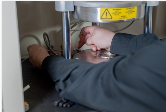
Reinstalling RTD in the Lower Platen
