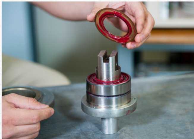
Removing Dust Cover and Inspecting Bearings
