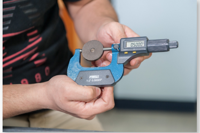
Measuring Rotor Dimensions with a Micrometer
