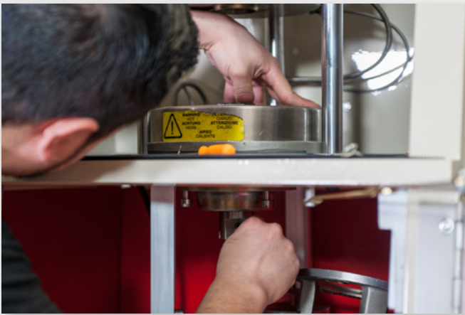
Using Rotor Height Gauge to Set Rotor Height
