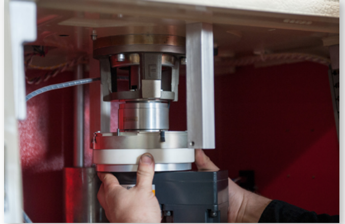
Removing Motor Drive Assembly
