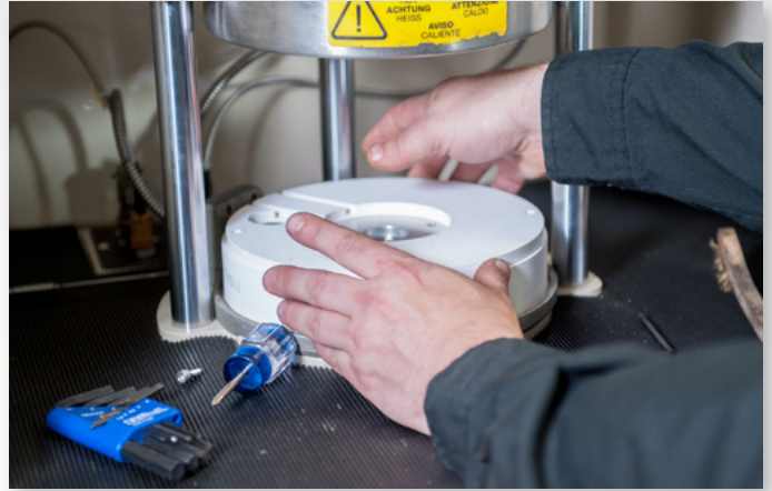
Removing Insulator from Lower Platen
