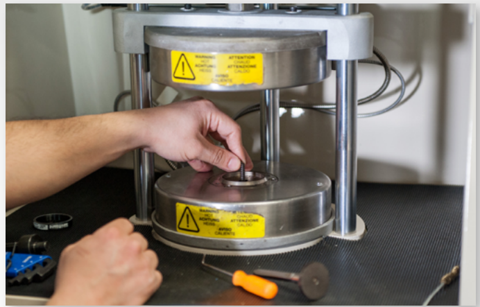
Reinstalling Rotor Height Spring
