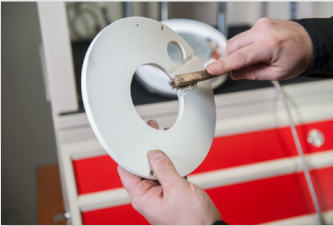
Cleaning Upper Platen Insulator
