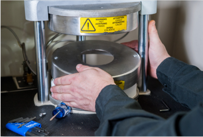
Disassembling Lower Platen
