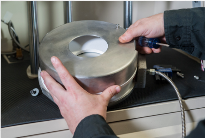
Reassembling Upper Platen
