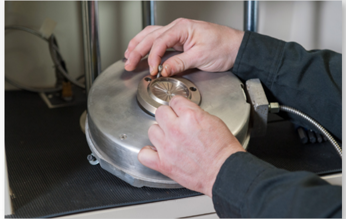
Removing Die from Upper Platen
