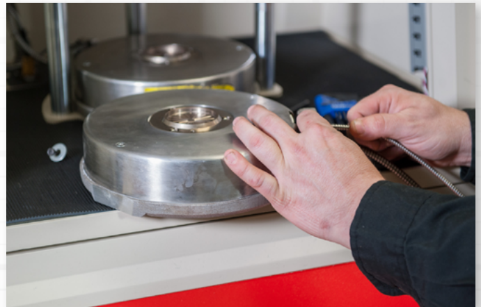
Reinstalling RTD in Upper Platen
