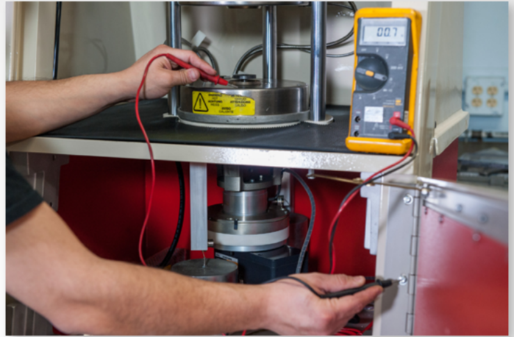
Checking Grounding on Lower Platen
