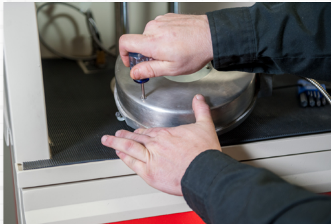
Disassembling Upper Platen
