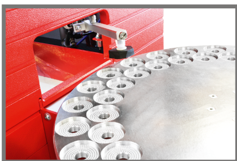
Automated MDR 3000. Robotic arm lifting test sample from tray to place onto die.
