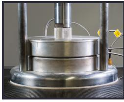
Platens closed for measurement of temperature.
