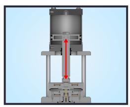
Cross-section of ODR platens and pneumatic cylinder.
