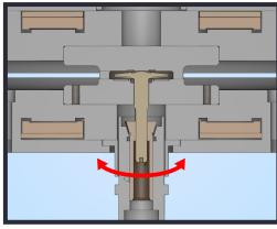
Cross-section of ODR test chamber. A motor/eccentric oscillates the central shaft and rotor to apply torsional force to the sample.
