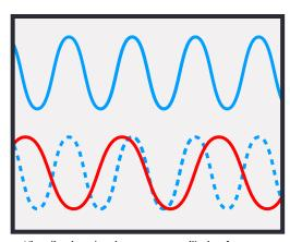
Visualization showing correct oscillation frequency (blue), overlaid on slower, incorrect frequency (red)
