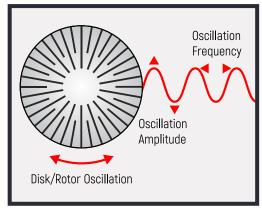
**Rotor Oscillation in an ODR:** Frequency and Amplitude of Oscillation shown as a sine wave.
